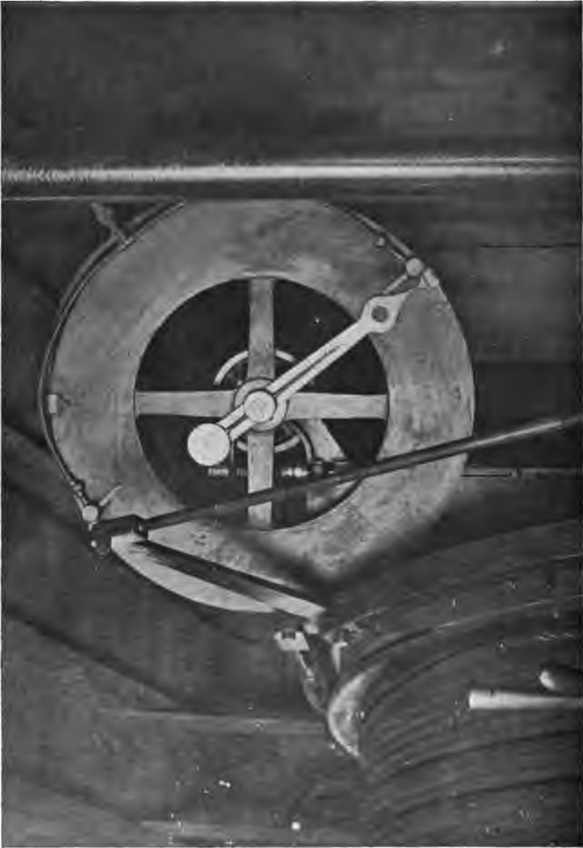
PLATE 84.—Overwinding Device on Dial of Hoisting Engine as Used on Shafts of Rondout Siphon. Hand trips small air valve which operates cut-off valve on air line to engine. Set so as to prevent cages from reaching top of head frames.
